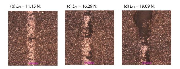
Fig. 2: The micro scratch track at different critical loads.
