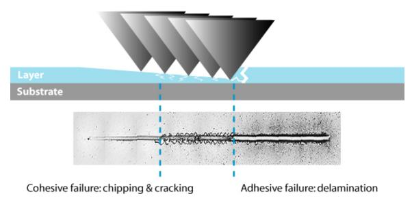
Fig. 1: Principle of scratch testing.
