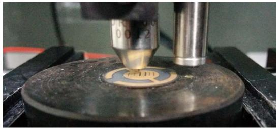
Fig. 1: Micro scratch tip and depth sensor on the QCM sample.
