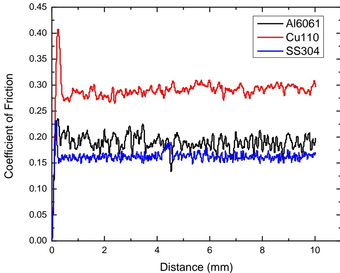
**Fig. 4: The evolution of coefficient of friction during the scratch hardness tests.**
