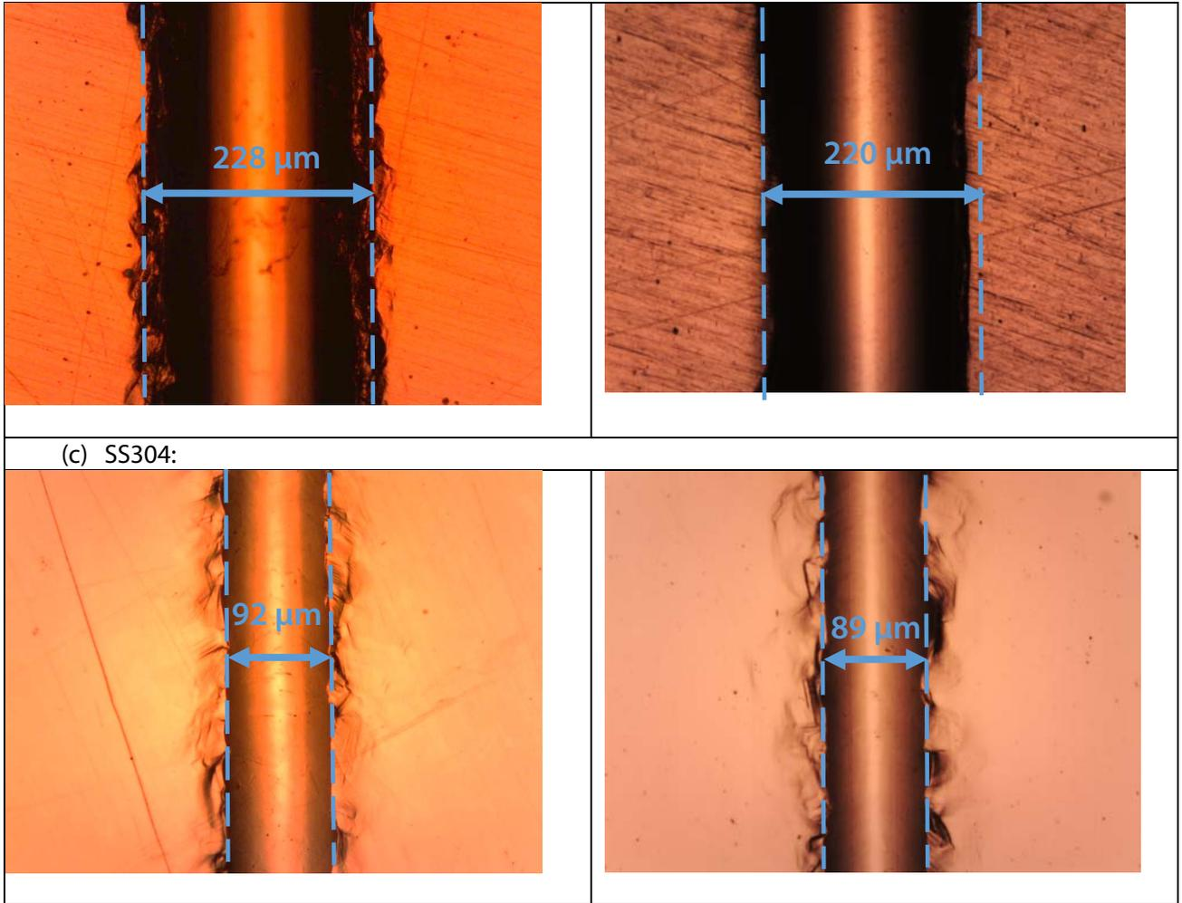
**Fig. 3: Scratch tracks under the microscope after the measurements (100X).**
