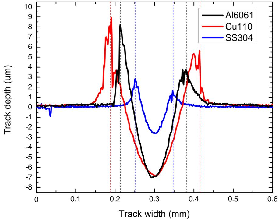
**Fig. 2: Scratch track profiles after the scratch hardness tests.**
