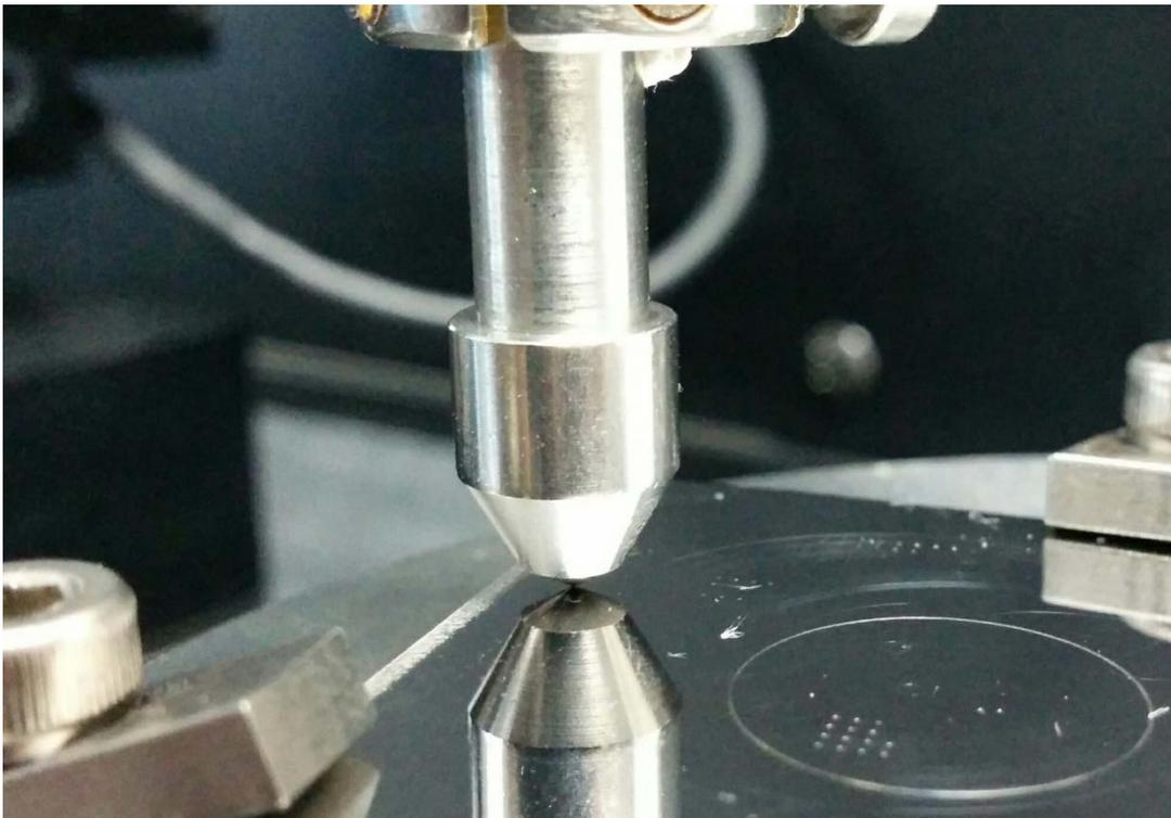
**Fig. 1: Scratch stylus on the test specimen.**
