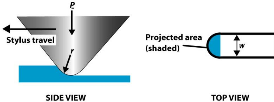
**Fig. 1: Schematic of scratch hardness measurement.**
