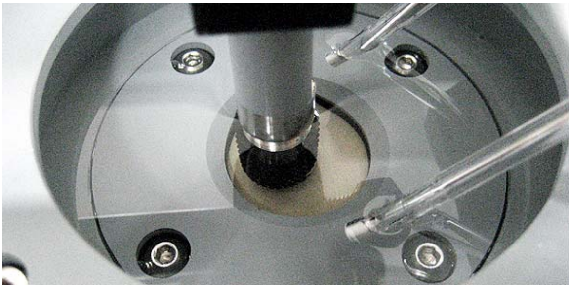
Fig. 1: Tribocorrosion module of the pin-on-disk tribometer.
