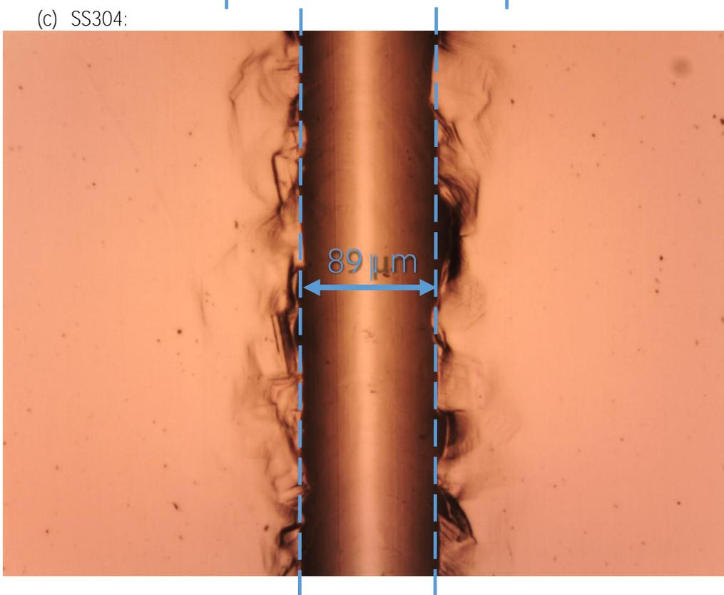
Fig. 3: Scratch tracks under the microscope after the measurements (100X).
