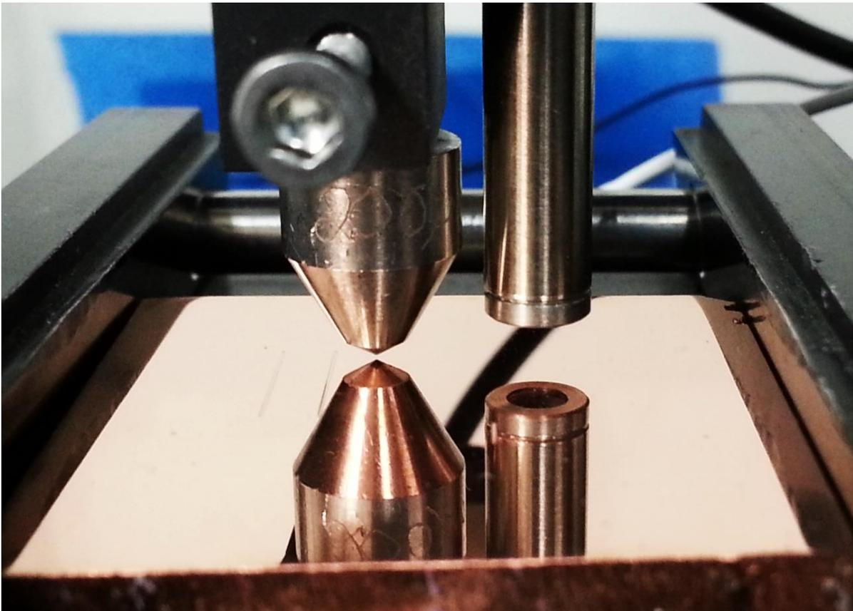
Fig. 1: Scratch stylus and depth sensor on the test specimen.
