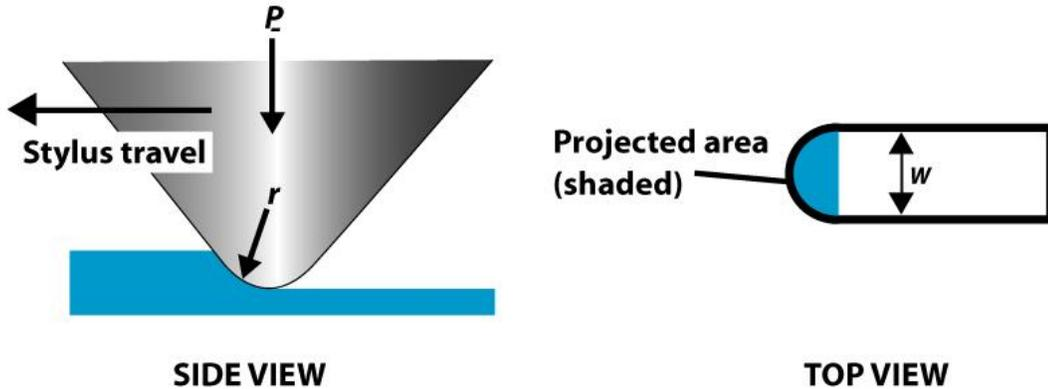
Fig. 2: Schematic of scratch hardness measurement.
