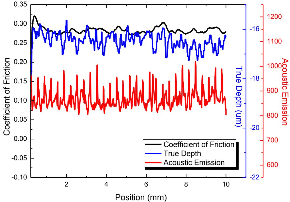
Fig. 4: The evolution of coefficient of friction, true depth and acoustic emission during the scratch hardness test on Cu110.
