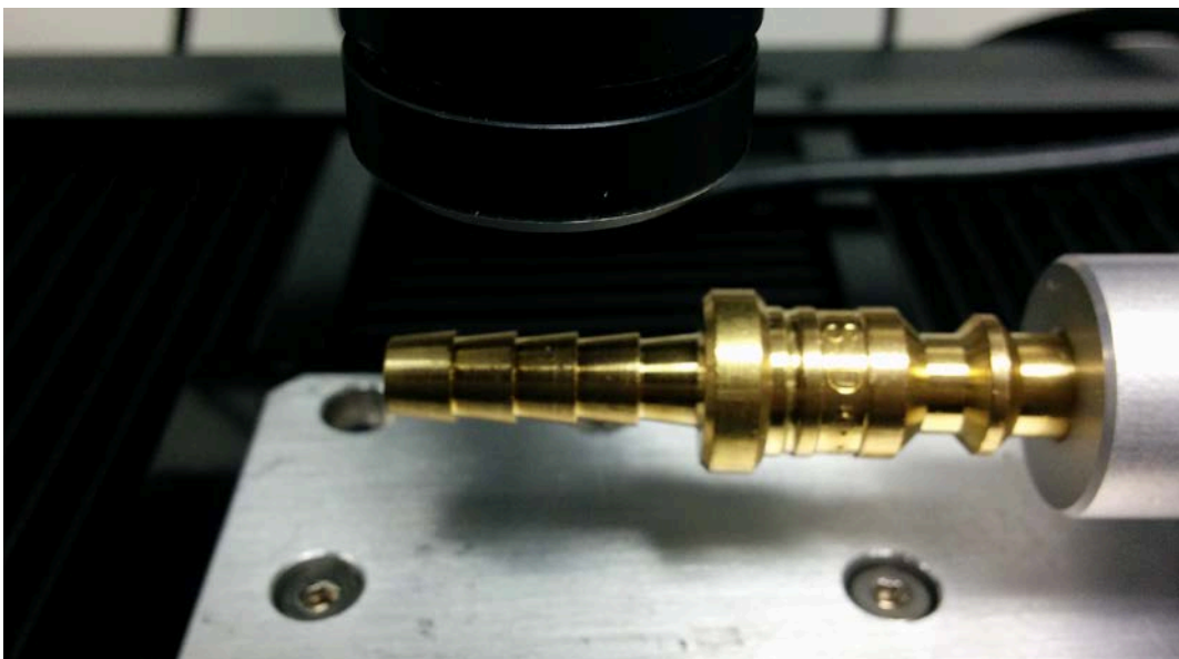
Fig. 1: Non-contact optical pen scanning on the sample.
