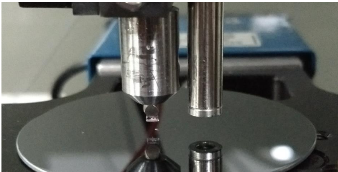
Fig. 1: Micro-scratch knife diamond tip and depth sensor on the polymer coating.
