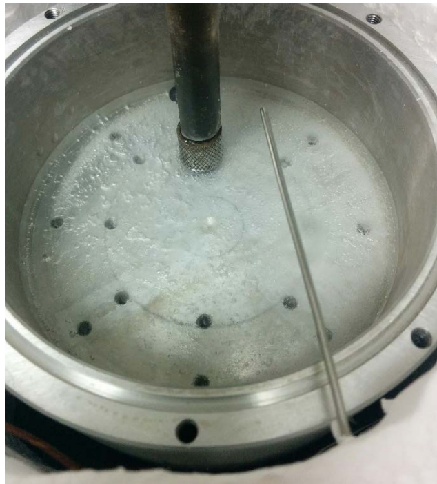
Fig. 1: Friction measurement of a rubber ball sliding on the ice surface.
