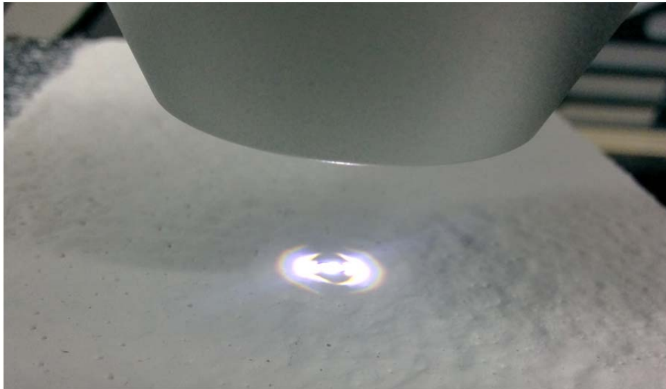
Fig. 1: Optical line-sensor scanning on the surface of the drywall sample.
