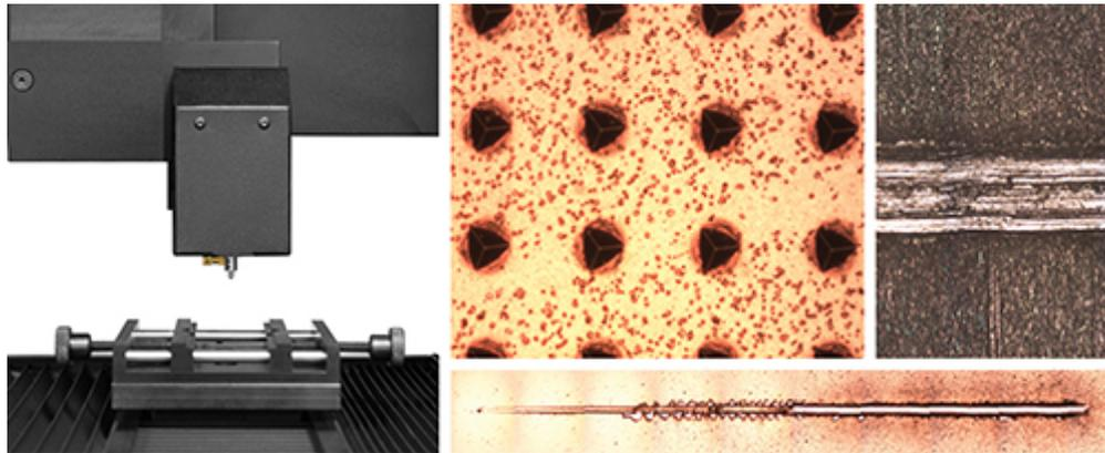
Nanovea Mechanical Tester's Micro Module is ideal for collecting local material properties on the surface of the sample. Insights on the relationships between microstructure to mechanical performance can be formed from the material properties each microstructure possess. This can provide information on the multifunctionality of the biological material and its benefits for the organism's survival in nature. These insights can also be used to help synthetically replicating biological materials.
