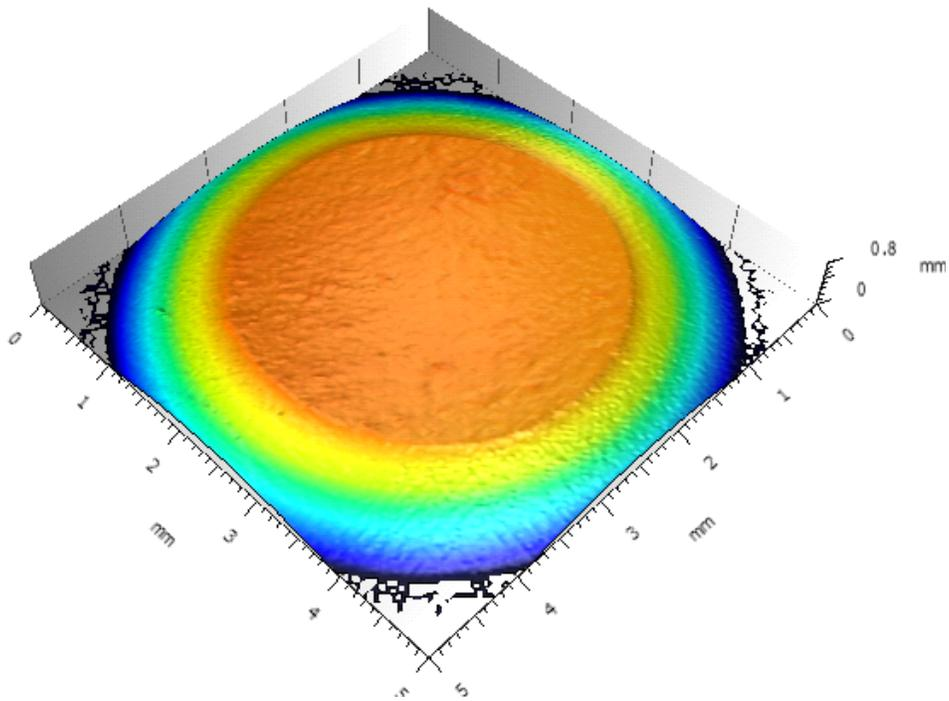
**Fig. 5: Wear scar on the Al<sub>2</sub>O<sub>3</sub> balls.**
