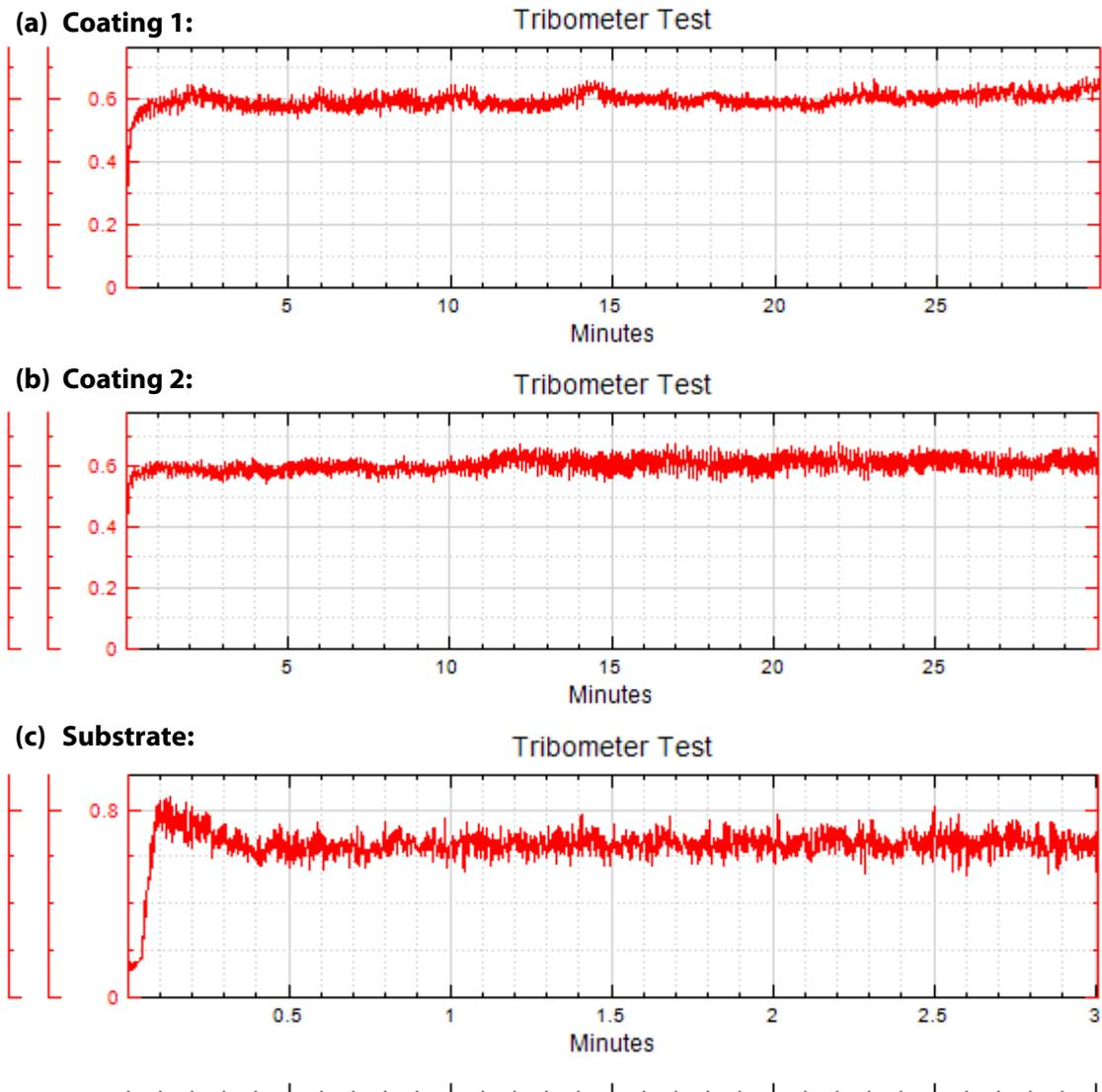
**Fig. 2: Evolution of COF during the wear tests. Note: The Substrate was tested for 3 min, compared to 30 min for the two Coatings.**
