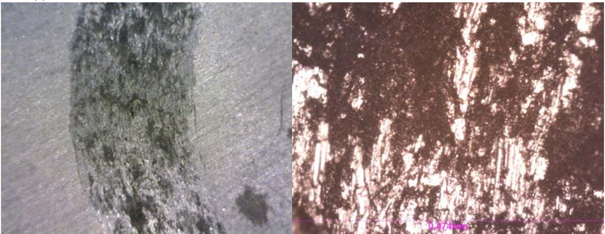
**Fig. 4: Wear tracks under optical microscope.**
