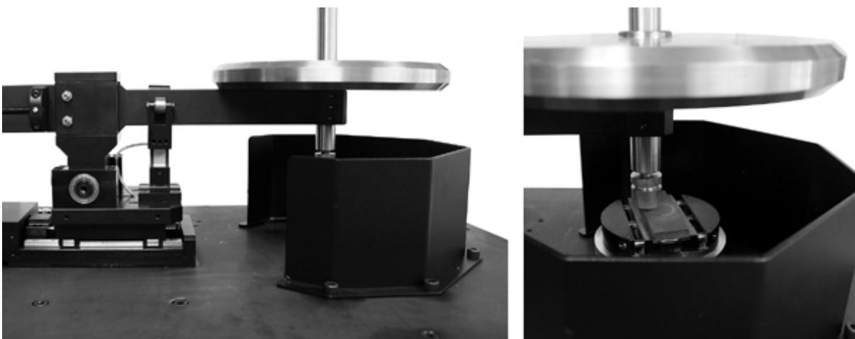
**Fig. 1: Setup of the high load wear test.**
