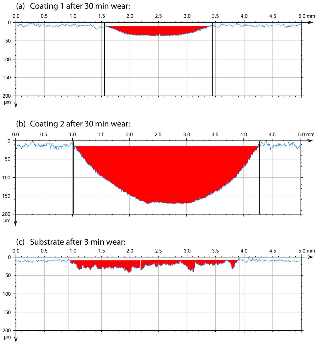
**Fig. 3: Wear tracks profiles after the tests.**
