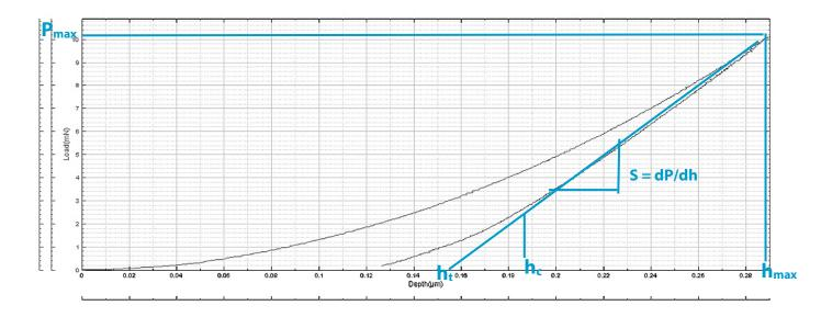
Fig. 6: Load-displacement curve of nanoindentation.
