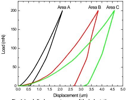
Fig. 4: Load-displacement curves of the indentations.
