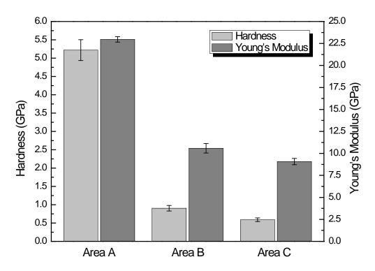
Fig. 5: Hardness and Young's Modulus at different locations of the PCB.
