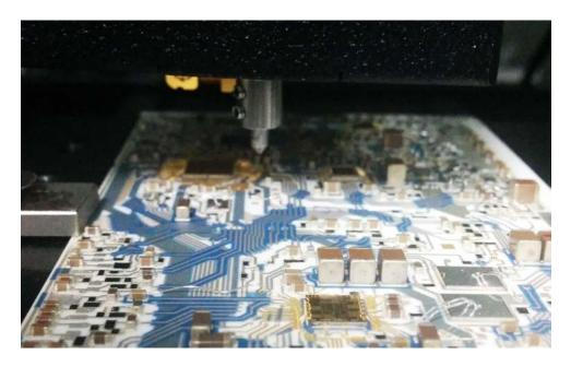
Fig. 1: Nanoindentation tip on the PCB.
