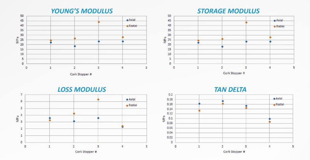
Between cork stoppers, the Young's modulus is not very different when tested in the axial orientation. Only Stopper #2 and #3 showed an apparent difference in the Young's modulus between the radial and axial direction. As a result, the storage modulus and loss modulus will also be higher in the radial direction than in the axial direction.
