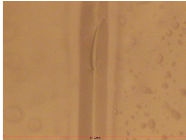
Figure 9 : Micrograph of Continuous Cracking – Aluminium 500x magnification (image width 0.102mm)
