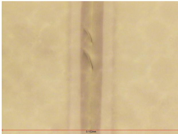
Figure 2 : Micrograph of the Initial Cracking – Glass 500x magnification (image width 0.102mm)
