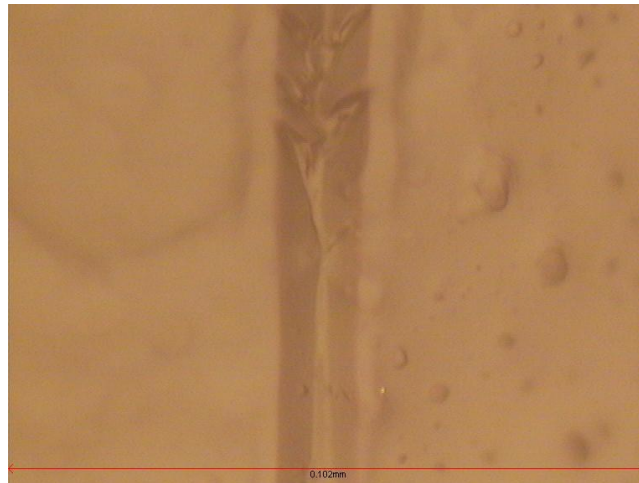
Figure 8 : Micrograph of the Initial Cracking – Aluminium 500x magnification (image width 0.102mm)
