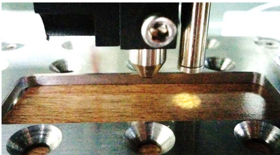
Fig. 1: Microindentation on a wood sample.
