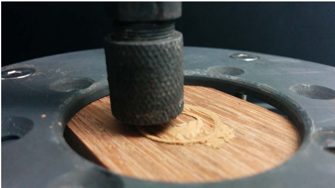
Fig. 1: Pin-on-disk wear test on the cherry wood sample.
