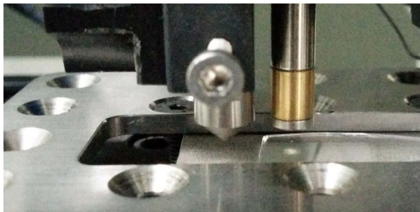
Fig. 2: Indentation of the SS304 sample.
