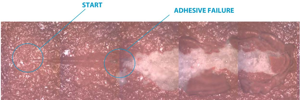
**Generic-** The critical load at which failure (delamination) occurred was 2.07N. Here we see the substrate exposed from delamination.
