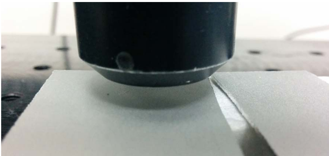
Fig. 1: Optical sensor scanning on the surface of the anodized aluminum sample.
