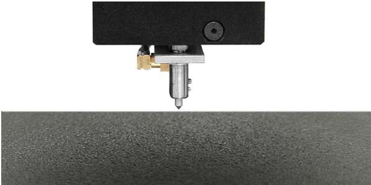
Fig. 1: Nano indenter on the shot peened surface.
