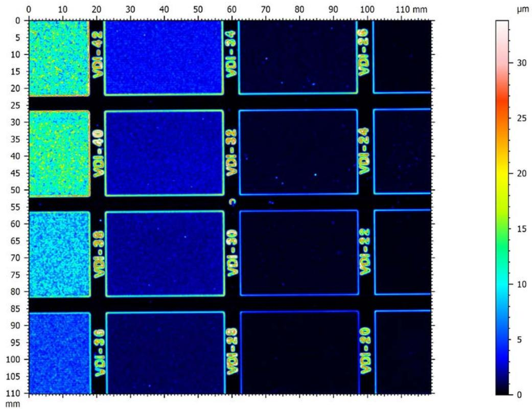
Fig. 2: False color views of the Surface Height Map and Roughness Distribution Map of the Roughness Standard Sample.
