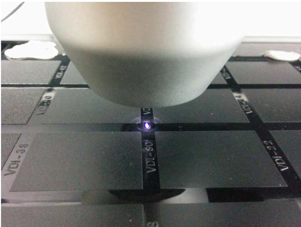
**Fig. 1: Optical line sensor scanning on the Roughness Standard sample.**
