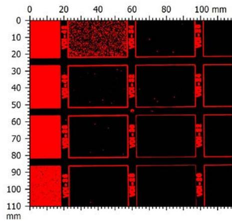
Fig. 3: Pass/Fail Map based on the Roughness Threshold.
