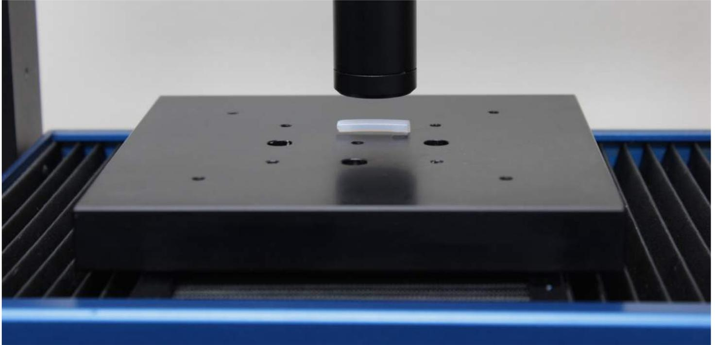
**Sample of catheter being analyzed with the Nanovea 3D Profilometer**
