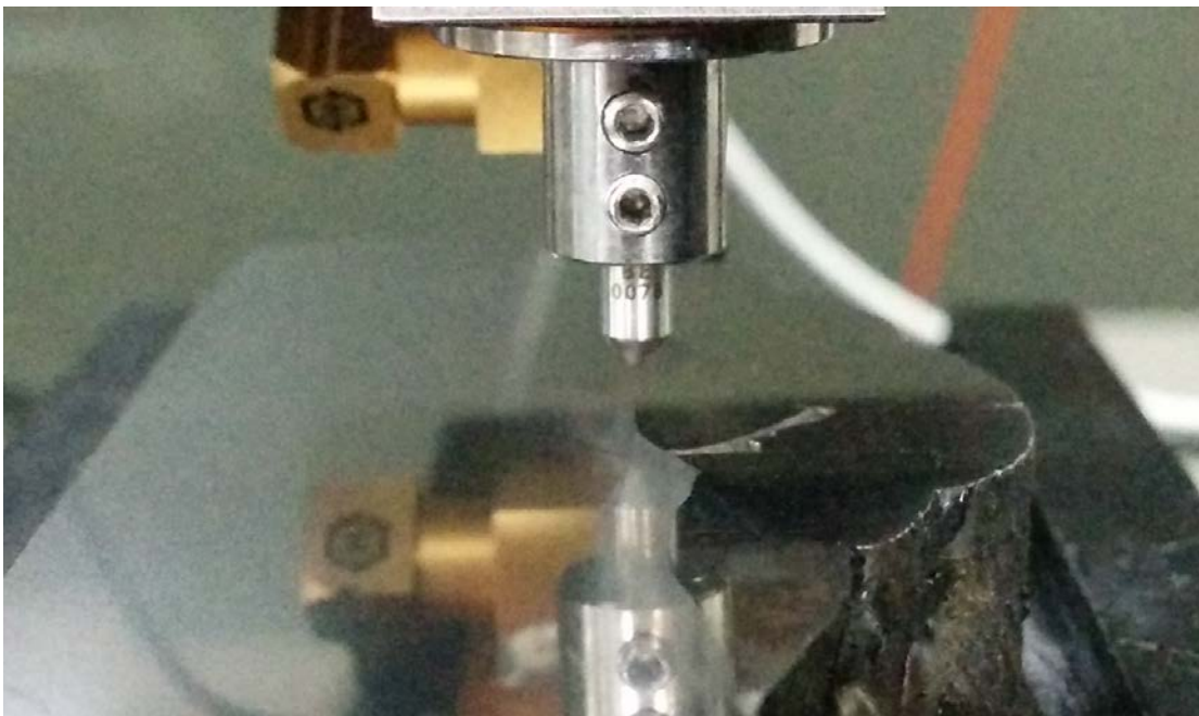
Fig. 1: Nanoindentation tip on the sample.
