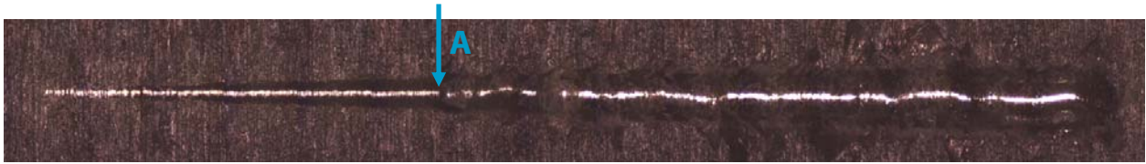
Fig. 5: Micrograph of full scratch of Sample A
