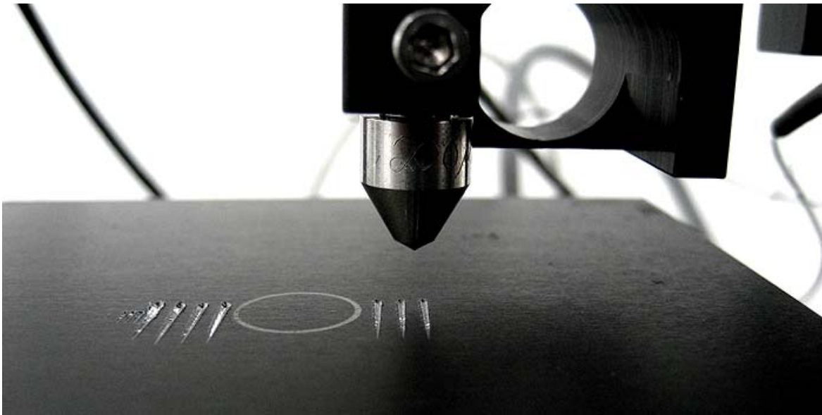
Fig. 1: Image of the indenter tip over the scratches of the tested sample
