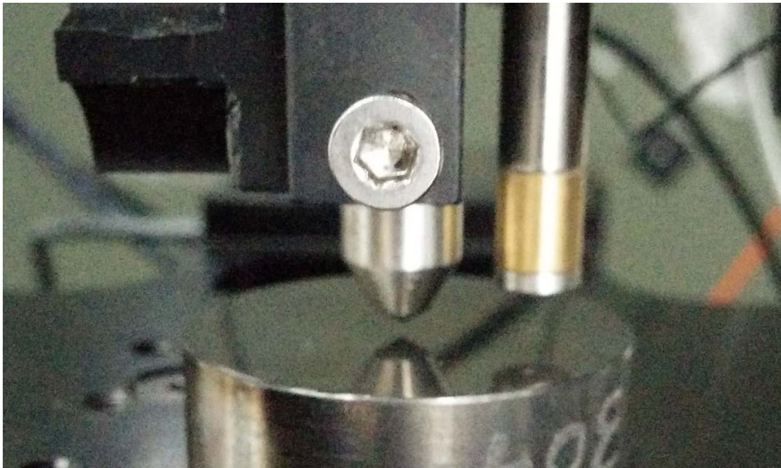
Fig. 1: Scratch tip on the DLC sample.
