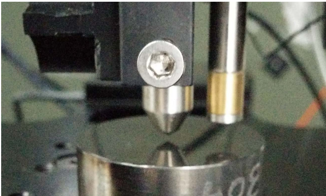
Fig. 1: Scratch tip on the DLC sample.
