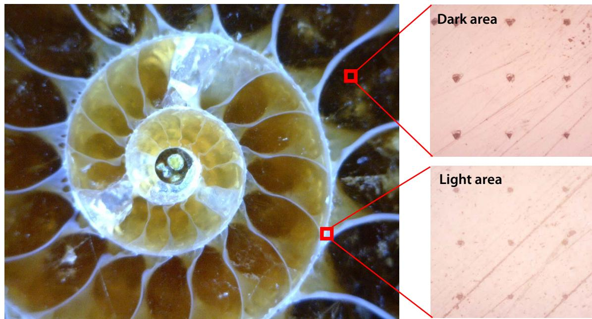
**Fig. 2: Location of indentations on the ammonite fossil sample.**
