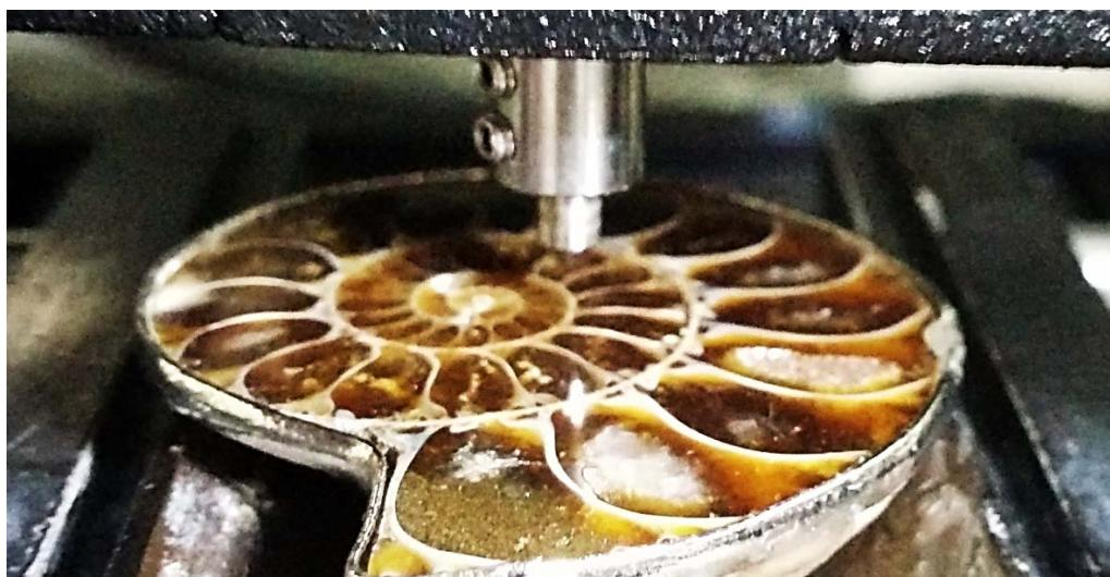
**Fig. 1: Nanoindentation tip on the ammonite fossil sample.**
