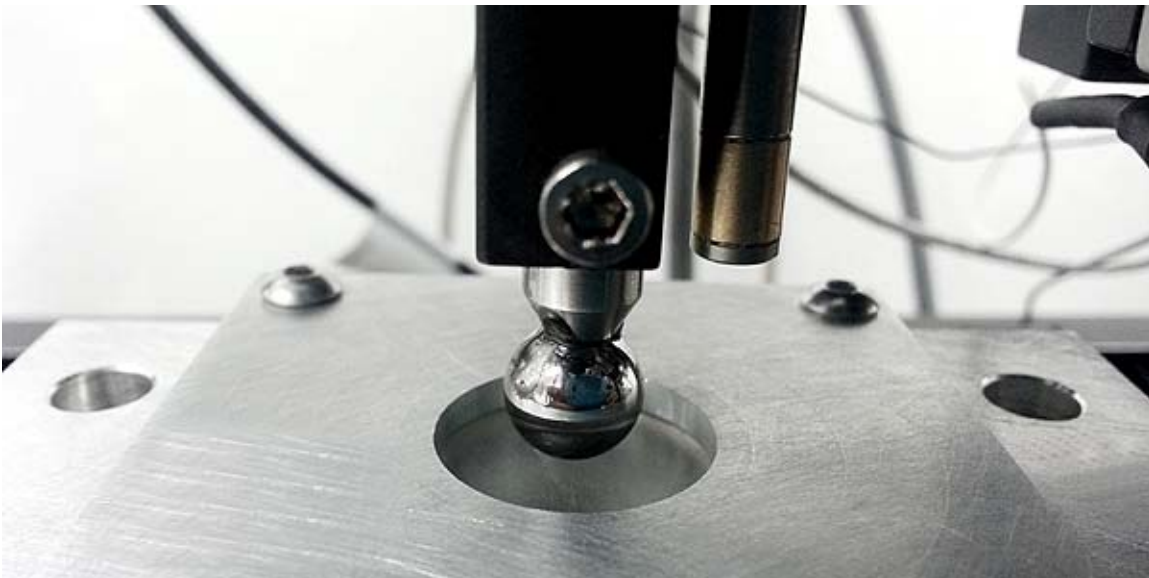
Fig. 1: The setup of the elastic/plastic property measurement on the polymer coating.
