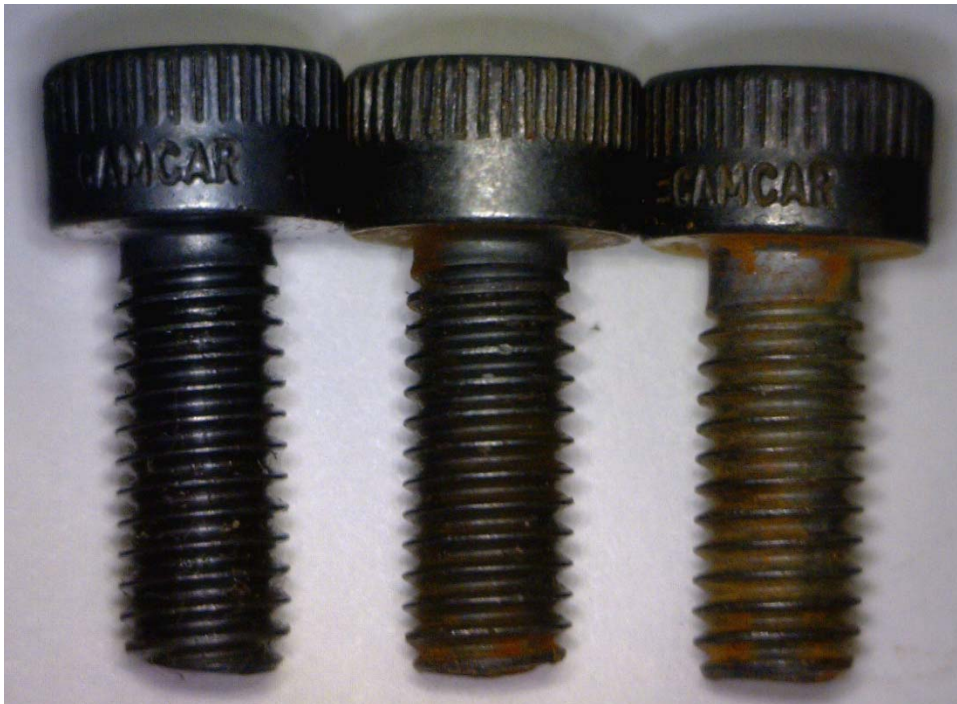
Fig. 5: Top and side views of the Alloy Steel screws before, and after 7 and 14 days corrosion tests (from left to right).
