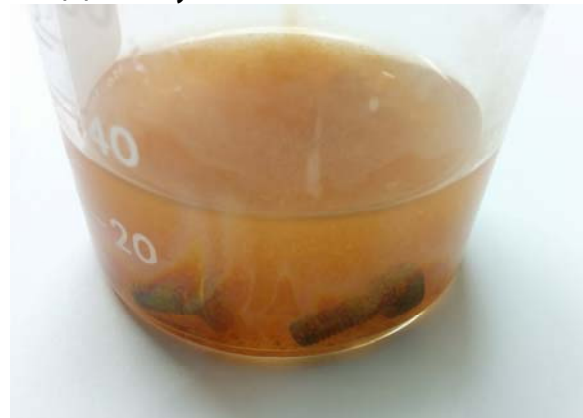
Fig. 4: The screws after 7 and 14 days immersion in the 3.5 wt. % NaCl solution.
