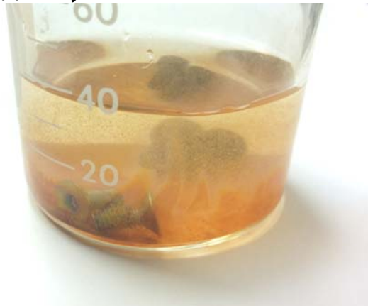
Fig. 4: The screws after 7 and 14 days immersion in the 3.5 wt. % NaCl solution.
