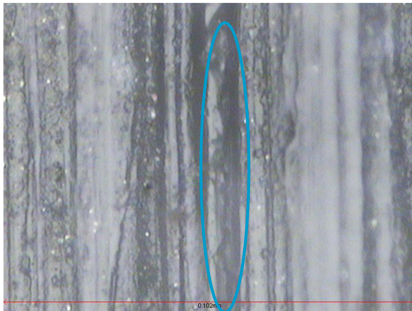
Micrograph of Initial Damage – SAMPLE 1, Scratch 3 500x magnification (image width 0.102mm)
