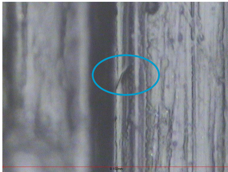
Micrograph of Initial Damage – SAMPLE 3, Scratch 2 500x magnification (image width 0.102mm)
