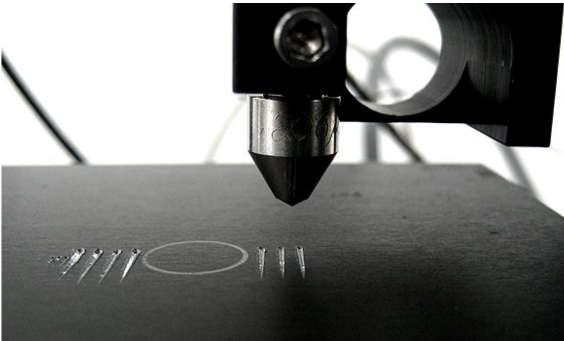
Fig. 1: Image of the indenter tip over the scratches of the tested sample.
