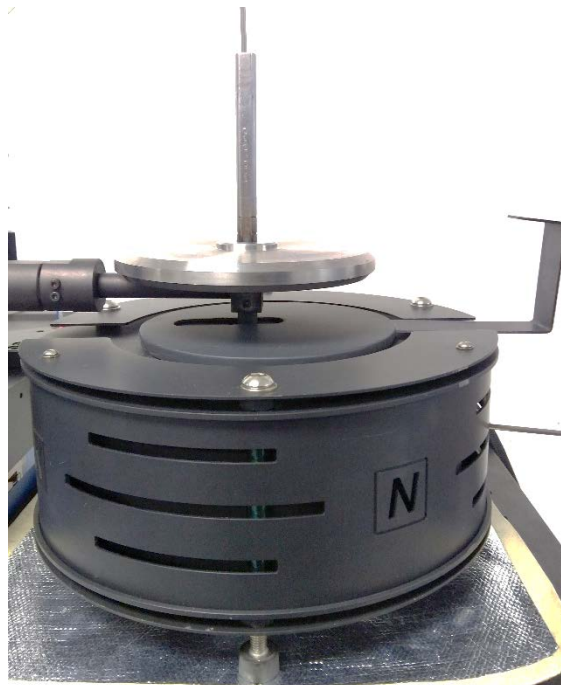
Figure 1: Tribology test setup for High Temperature Brake Pad Tests
