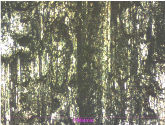
Fig. 3: Wear scars of the blocks after (a) dry and (b) lubricated wear tests.
