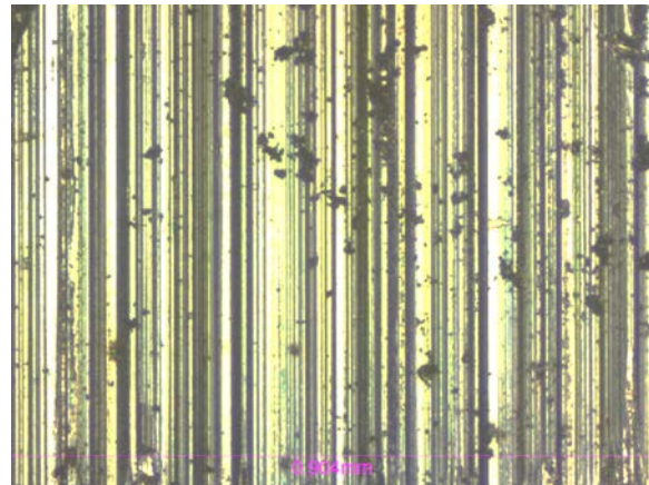
Fig. 3: Wear scars of the blocks after (a) dry and (b) lubricated wear tests.
