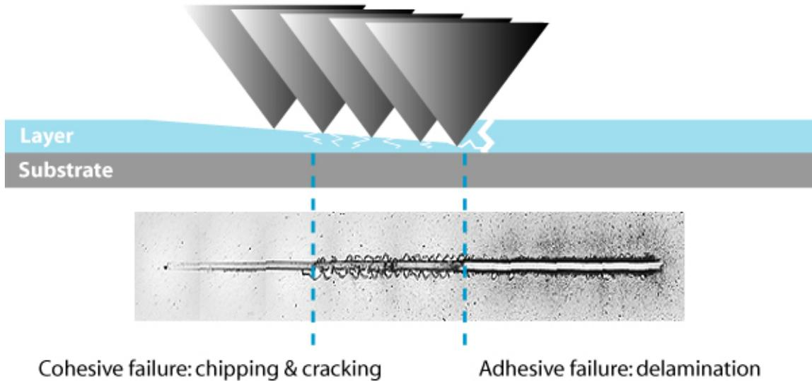
**Fig. 1: Principle of scratch testing.**
