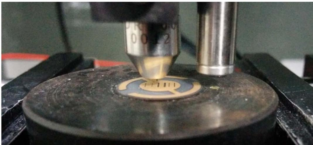
**Fig. 1: Micro scratch tip and depth sensor on the QCM sample.**
