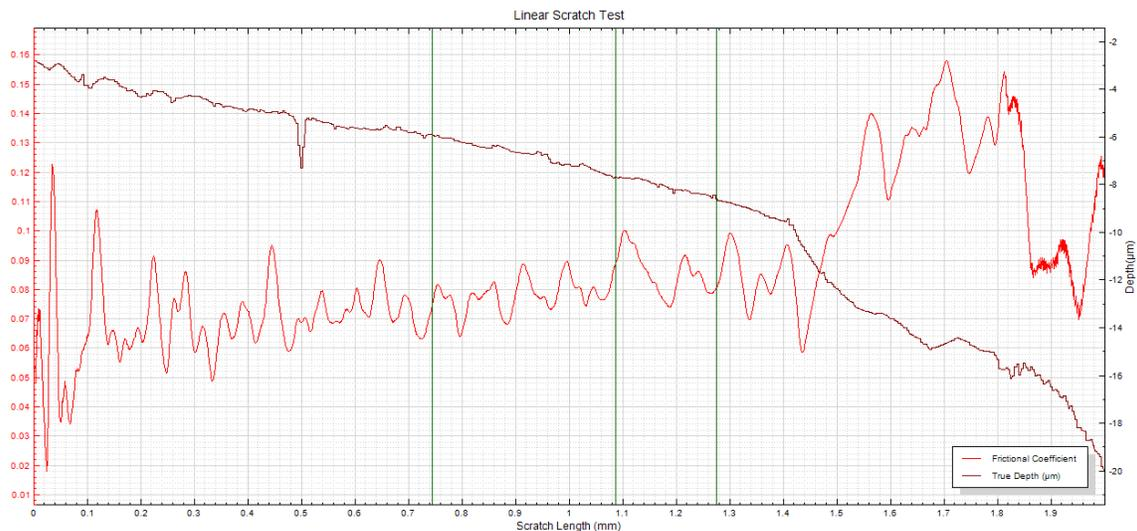
**Fig. 3: Evolution of friction coefficient and depth during the micro scratch test.**
