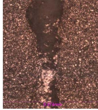
**Fig. 2: The micro scratch track at different critical loads.**
