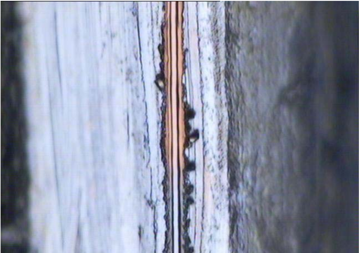
Figure 2 : Micrograph of Failure – Tin Coating 500x magnification (image width 0.0615mm)
