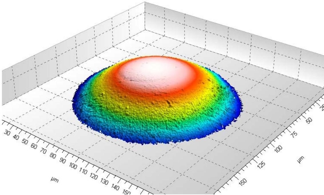
Surface shape removed and roughness values calculated
