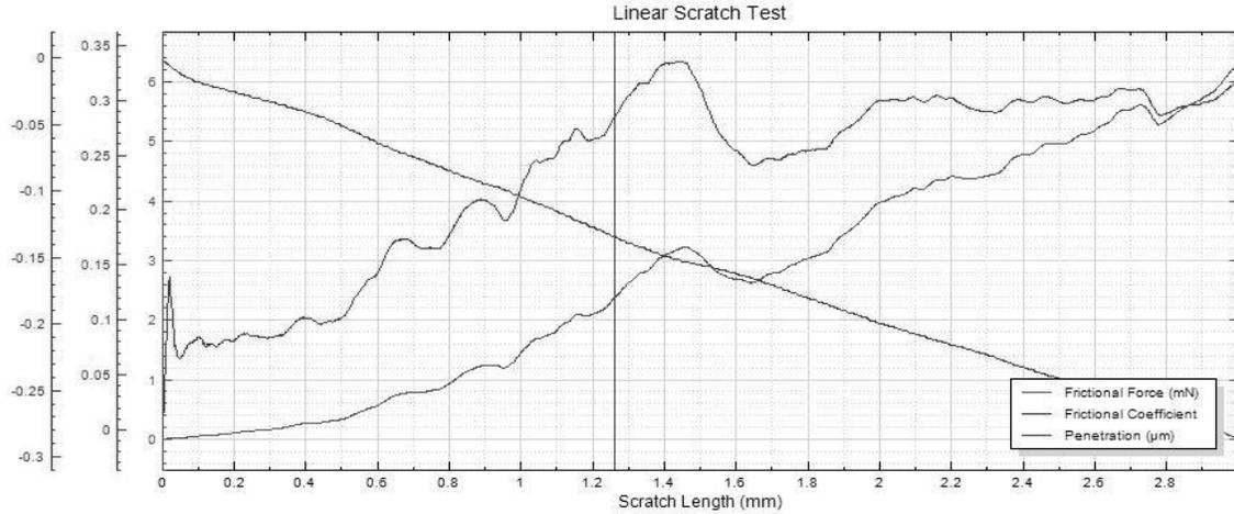
**Fig. 8: Friction graph showing line of critical point of failure - PTFE.**
