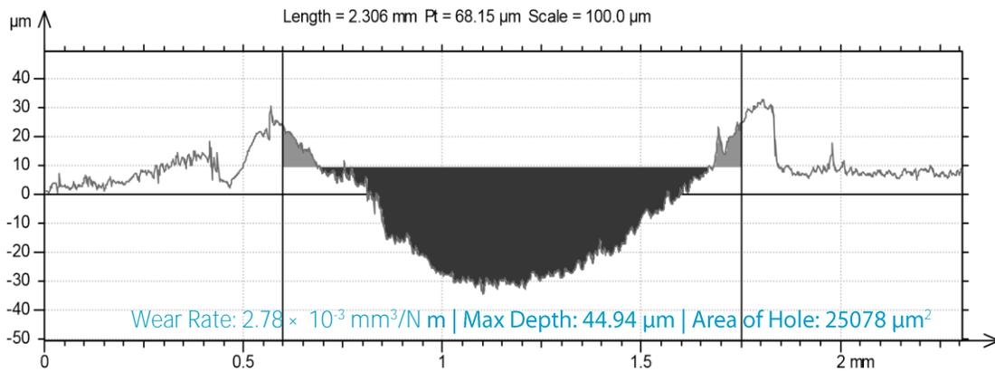
**Fig. 5: Profile extraction of wear track – PTFE.**
