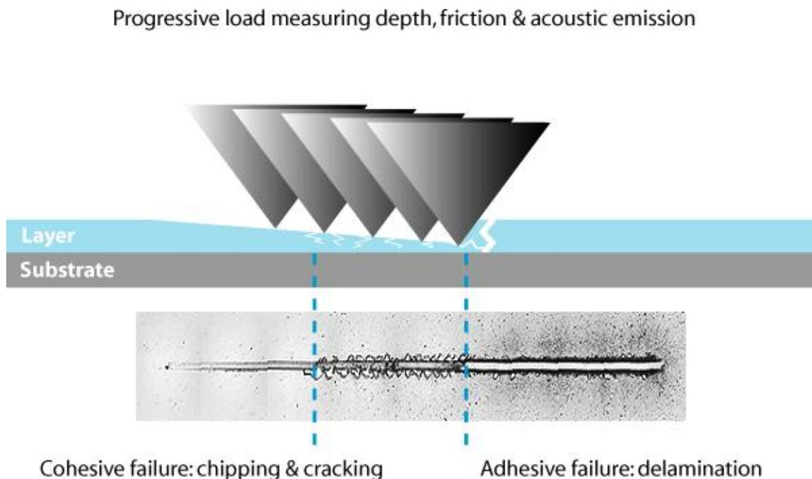
**Fig. 3: Principle of scratch testing.**
