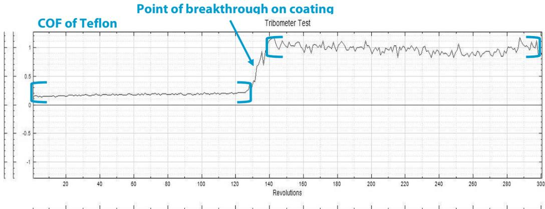
**Fig. 4: Evolution of COF of PTFE coating during wear.**
