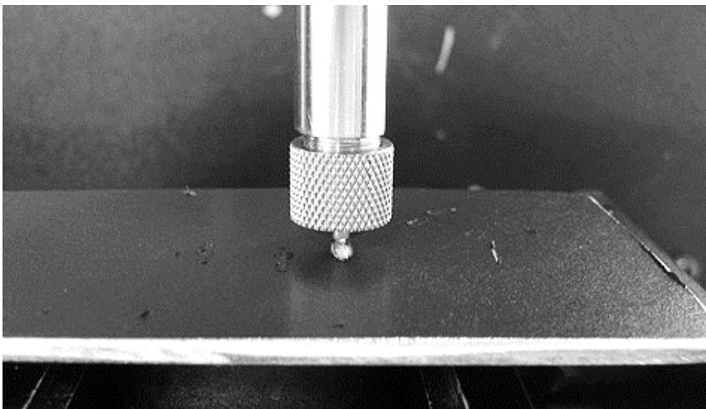
**Fig. 1: Setup of linear reciprocating wear test using Nanovea Tribometer.**
