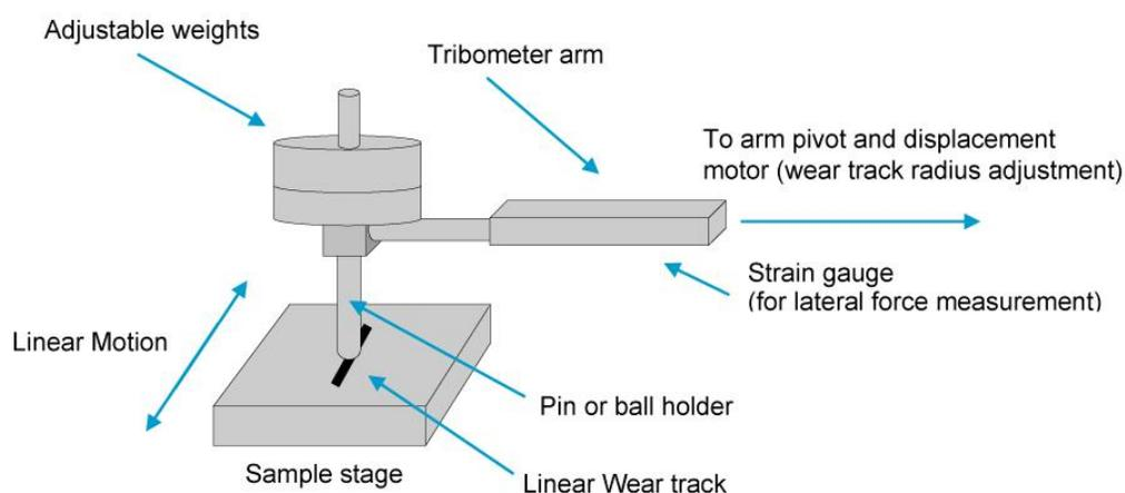
**Fig. 2: Schematics of linear reciprocating wear test.**
