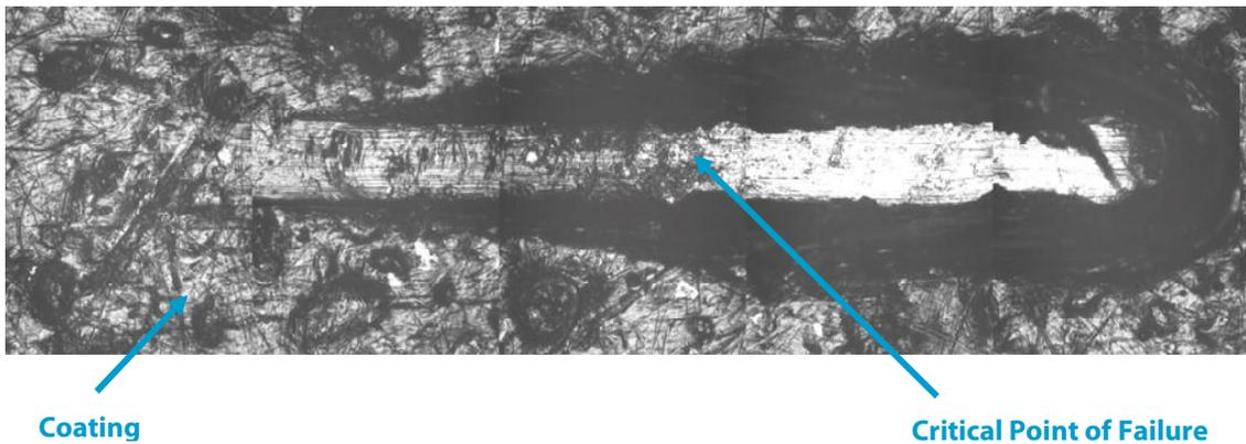
**Fig. 6: Micrograph of full scratch on PTFE (10X).**
